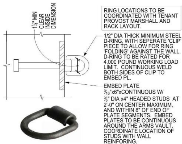
ENLARGED STEEL RING ASSEMBLY DETAIL
